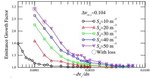
Figure 6: (Color) EGF across octupole driven resonance  $4\nu_{z0} = 27$  versus tune-ramp rate for various octupole strengths after 70-turn injection. Linear relationships are evident.
