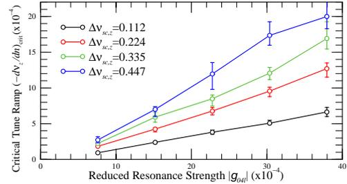
Figure 7: (Color) Critical tune-ramp rate across the octupole driven resonance  $4\nu_{z0} = 27$  versus reduced resonance strength  $|g_{04\ell}|$  for various bunch intensities.
