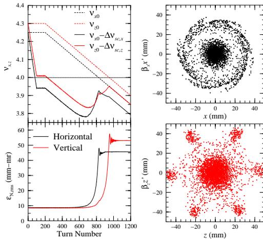
Figure 2: (Color) Top-left: After 100-turn injection, bare tunes are ramped downwards at  $-0.004$  per turn. Systematic resonances  $6\nu_{x0,z0} = P$  are crossed at turns 950 and 825, respectively. Bottom-left: Emittance growths are observed. Right: Horizontal and vertical phase-space distributions at turn 900.
