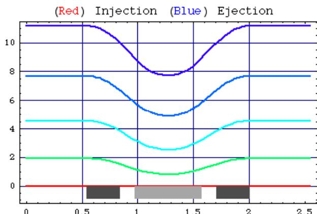
Figure 4: Closed Orbits during the Acceleration Cycle.
