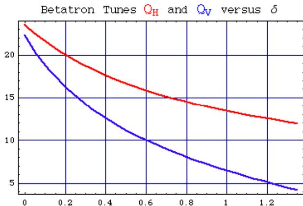
Figure 3: Betatron Tunes during the Acceleration Cycle.
