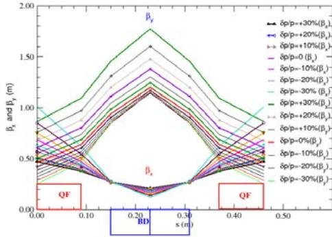
Figure 2: Betatron functions  $\beta_x$  and  $\beta_y$  in the basic cell.
