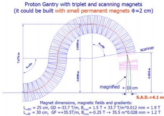
Figure 3: Proton permanent magnet NS-FFAG gantry.
