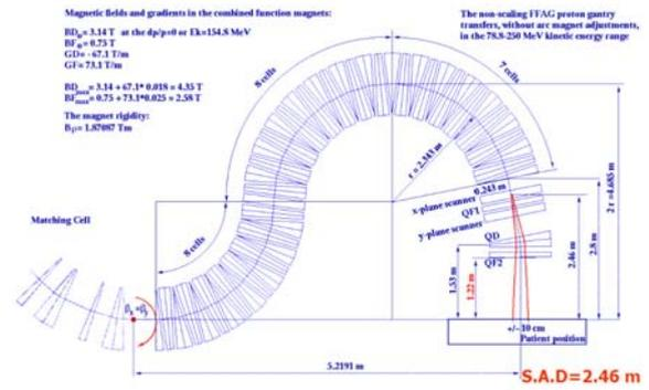
Figure 4: The superconducting proton gantry.
