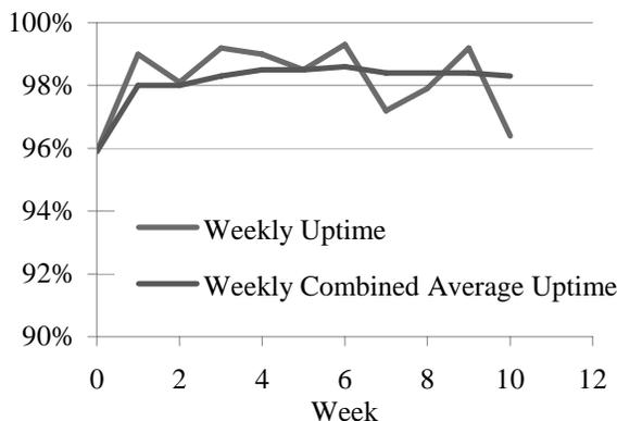
Figure 5: TR30/2 1.2mA Uptime Test
