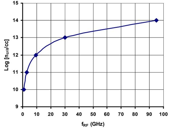
Figure 1: Critical plasma density vs. RF frequency plot.
