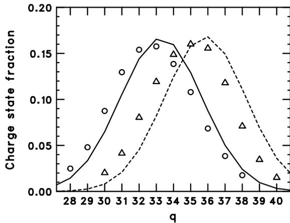
Figure 2: Charge state distributions of uranium at 0.67 and 0.87 MeV/nucleon behind a 20- $\mu\text{g}/\text{cm}^2$ -thick carbon foil. The horizontal and vertical axes indicate the charge state and charge state fraction of uranium ions, respectively. Circles and triangles represent the data measured at 0.67 and 0.87 MeV/nucleon, respectively. Solid and dashed lines represent the values from the table in ref. [5] at 0.67 and 0.87 MeV/nucleon, respectively.
