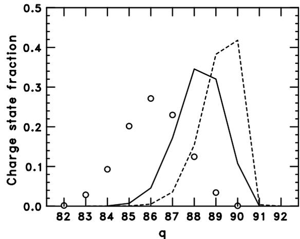
Figure 6: Charge state distributions of uranium at 51 MeV/nucleon stripped by 14-mg/cm<sup>2</sup>-thick carbon foil. The horizontal and vertical axes indicate the charge state and charge state fraction, respectively. The circles, solid line, and dashed line represent the measured data, GLOBAL calculation, and ETACHA calculation, respectively.
