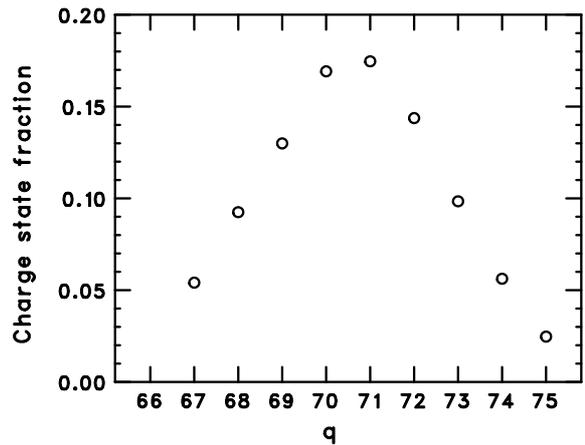
Figure 4: Charge state distribution of uranium at 11 MeV/nucleon stripped by 0.3- $\text{mg}/\text{cm}^2$ -thick carbon foil. The horizontal and vertical axes indicate the charge state and charge state fraction of uranium ions, respectively.
