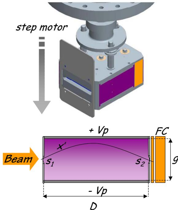
Figure 2: NSCL Allison-type emittance scanner. See text for details.
