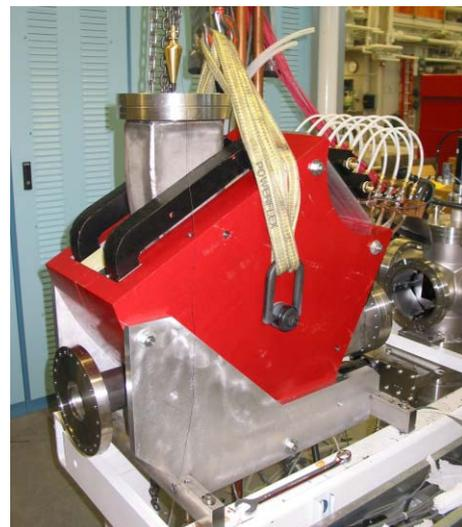
Figure 9: New analyzing magnet installed under Artemis-B in July 2007. The port on the left can be used for pumping.
