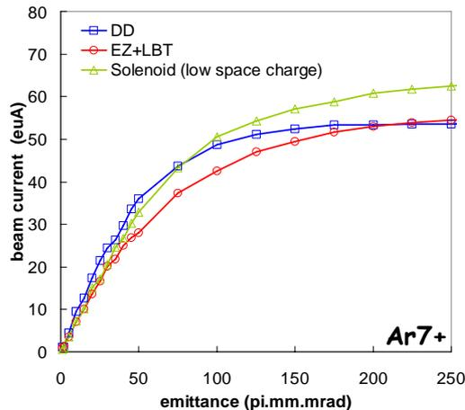
Figure 8: Beam brightness for the two electrostatic systems currently used under the production ECR sources at the CCF. The beam brightness for the solenoid system with low space charge effects is also given for comparison. All cases are for a 20 kV  $^{40}\text{Ar}^{7+}$  beam from Artemis-B.
