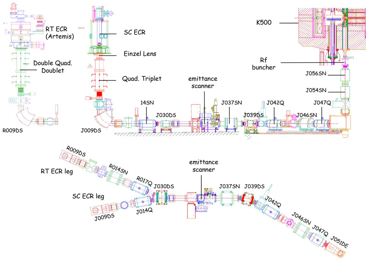
Figure 1: Layout of the CCF beam injection line. Side view of RT ECR (upper left), side view of SC ECR and injection line (upper right) and top view of injection line (bottom). Magnetic focusing solenoids were replaced by electrostatic focusing systems under both ECR sources to avoid possible space charge effects. After the charge state selection, magnetic and electrostatic elements are used for focusing.
