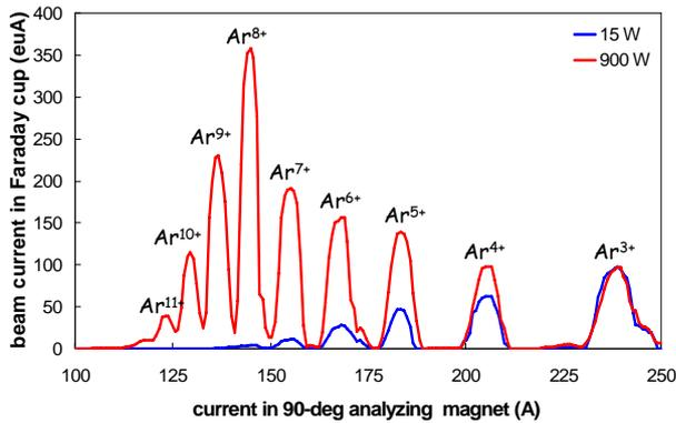
Figure 3: Charge State Distribution (CSD) for Argon beam measured on Artemis-B for 15 W and 900 W of rf microwave power injected into the ECR plasma.
