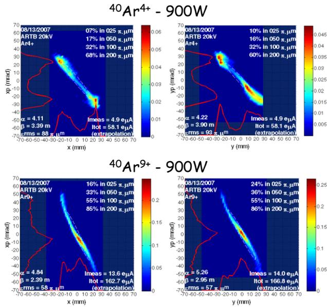
Figure 6: Transverse emittances for  $\text{Ar}^{4+}$  and  $\text{Ar}^{9+}$  beams for the 900 W case. The  $\text{Ar}^{4+}$  emittances are hollow while the  $\text{Ar}^{9+}$  emittances are centered on a core. For the 15 W case no hollow emittances could be observed.
