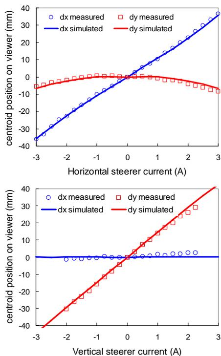
Figure 10: Simulated and experimental beam centroid response curves to horizontal (top) and vertical (bottom) deflection from a steerer located upstream of the new analyzing magnet. The centroid is measured on a beam viewer downstream of the analyzing magnet.
