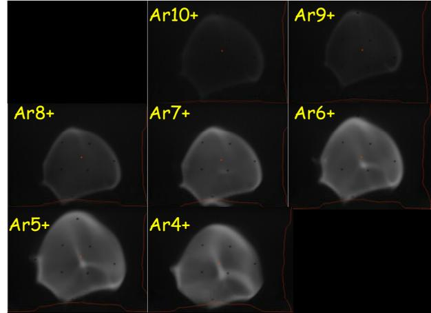
Figure 4: Pictures of the different charge states of an Argon beam on a beam viewer located one meter after the analyzing magnet for the 15 W case.
