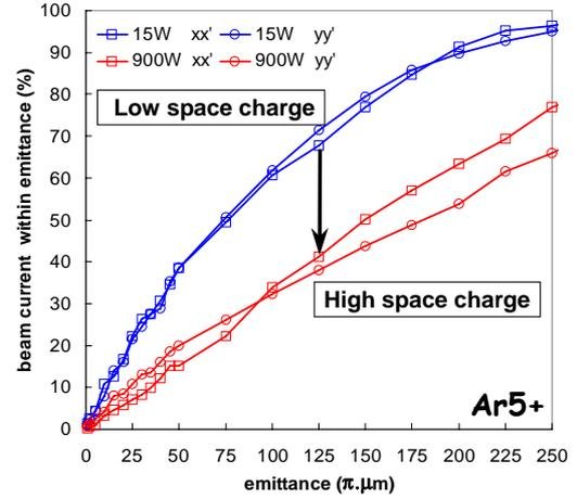
Figure 7: Transverse beam emittances for  $\text{Ar}^{5+}$  beam and for the two different cases of microwave power. For the low power case, the space charge forces are small and have a negligible effect on the beam brightness. In the high power case, the space charge forces are significant and the brightness is degraded.
