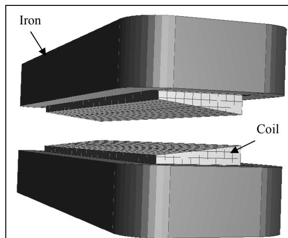
Figure 2: Model of Active Magnetic Channel
