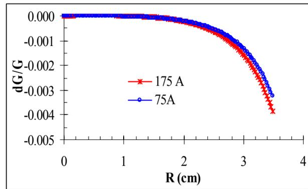
Figure 7: Field Homogeneity Profile at different excitations
