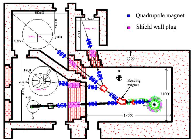
Figure 10: External Beam handling system layout with building
