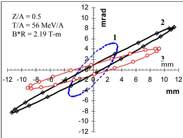
Figure 4. Radial phase space ellipse of same beam at (1) M9\_Slit (2) at common point without M9 channel (3) at common point in presence of M9 channel.
