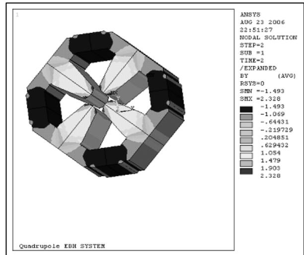
Figure 6: Magnetic Field Contour in ANSYS-3D for B-Type Quadrupole
