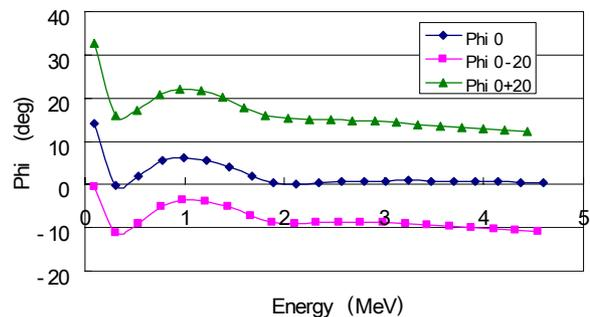
Figure 1: the phase history of particles as a function of energy starting with three initial RF phases, the graph was plotted at the center line of the first dee ( $\theta=0^\circ$ )
