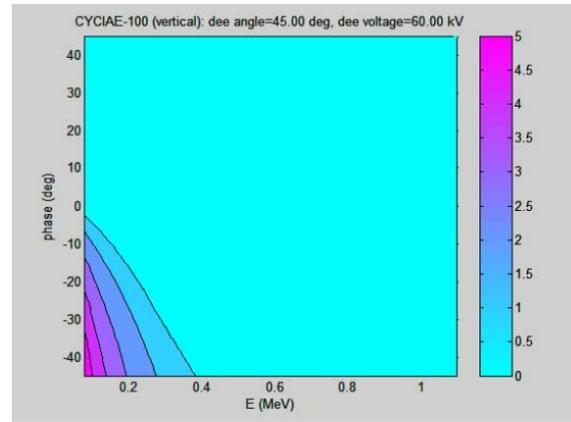
Figure 5: The contour plot for imaginary part of the vertical tune
