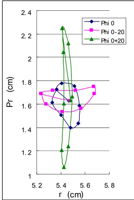
Figure 2: the radial phase results, corresponding to three RF phases, from the eigen-ellipses ( $\sim 1.89\text{MeV}$  for Phi0) with  $0.5\text{ pi-mm-mrad}$  emittance tracking backwards to the injection point ( $0.04\text{MeV}$ )
