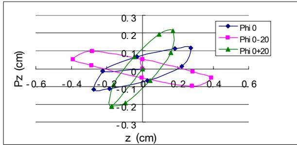
Figure 3: the vertical results, corresponding to three RF phases, from the eigen-ellipses ( $\sim 1.89\text{MeV}$  for Phi0) with  $0.5\text{ pi-mm-mrad}$  emittance tracking backwards to the injection point ( $0.04\text{MeV}$ )
