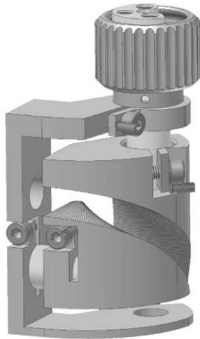
Figure 3: The spiral inflector, with the bayonet type connection.
