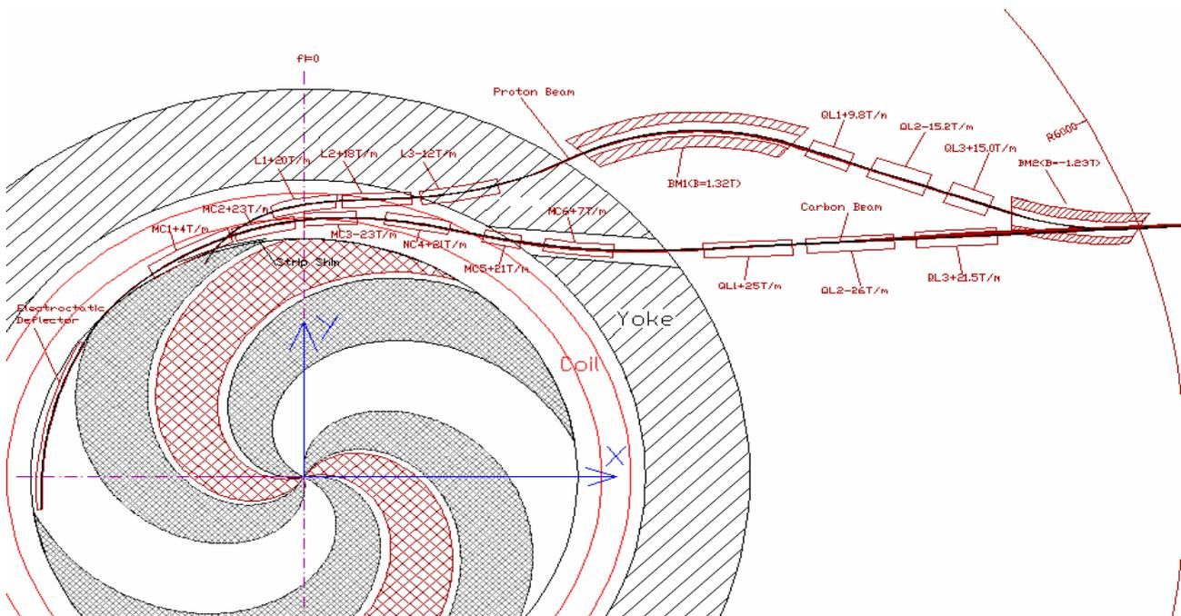
Figure 4: Plan view of the carbon and proton extracted beams and of the elements of extraction lines (proton beam is shown from the pole edge).
