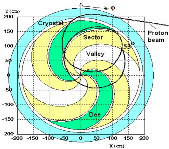
Figure 3: Extraction trajectory of the 260 MeV proton beam.
