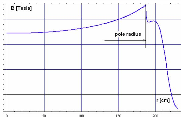
Figure 1: Average magnetic field of C400 cyclotron.
