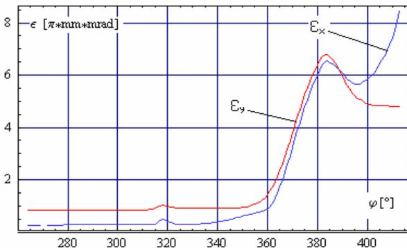
Figure 8: RMS emittances of the carbon beam during the extraction in the cyclotron (final point of computation is located at exit from the return yoke)
