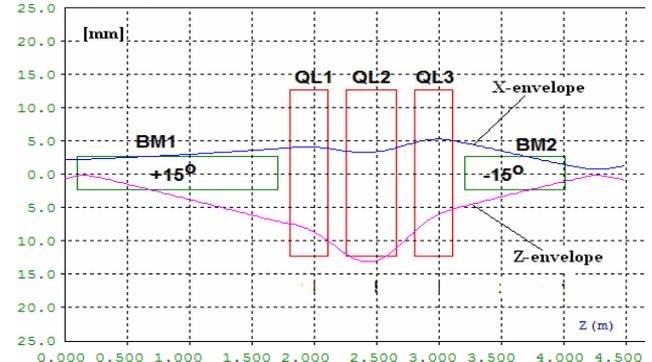
Figure 10: Proton beam RMS envelopes outside the cyclotron. Z is a length of the beam way from the entrance into the first Bending Magnet.
