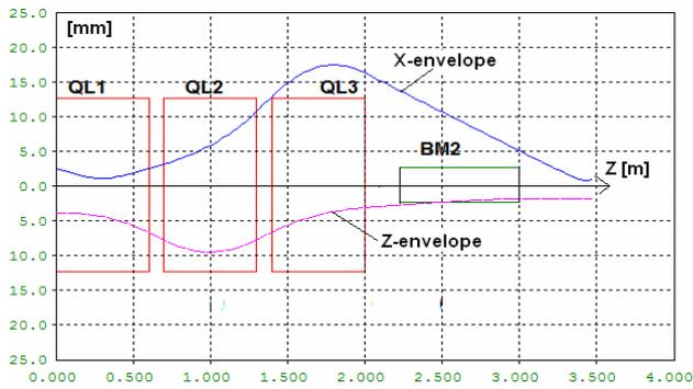
Figure 6: RMS carbon beam envelopes outside the cyclotron. Z is a length of the beam way from the entrance into the first lens QL1.
