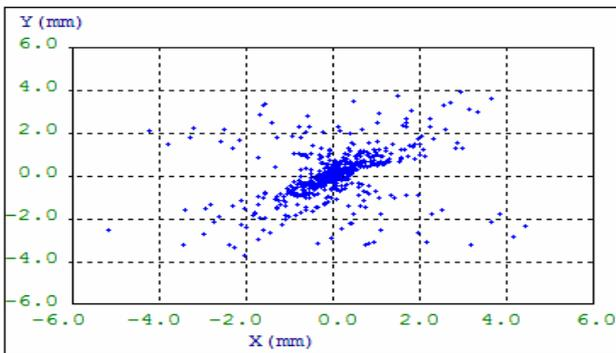
Figure 7: Carbon beam portrait on transverse plane just before the energy degrader.
