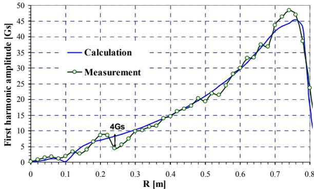
Figure 4: The calculation and measured form of the first harmonic amplitude at the case of the sector shims installation, but without the magnetic channel.
