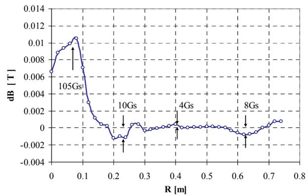
Figure 3: The deviation of the measured average magnetic field from the calculation results, 1.43T
