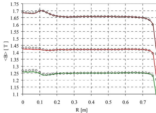
Figure 2: The calculation form of the average magnetic field (circles) and the results of the measurements (line)
