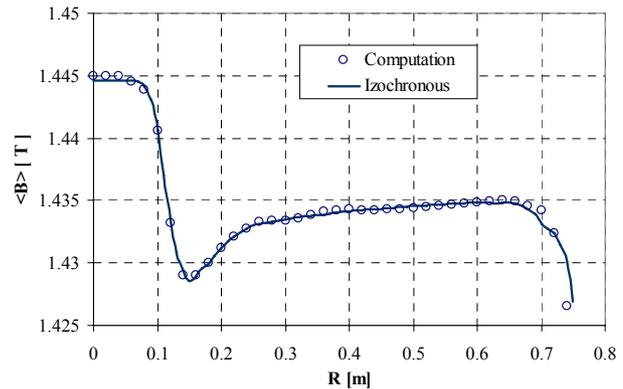
Figure 1: The isochronous magnetic field and the result of numerical formation.
