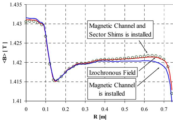
Figure 5: The form of the average magnetic field at the case of: isochronous distribution; with installation magnetic channel only; with installation both magnetic channel and sector shims.
