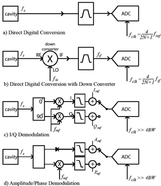
Figure 1. Difference Demodulation Schemes
