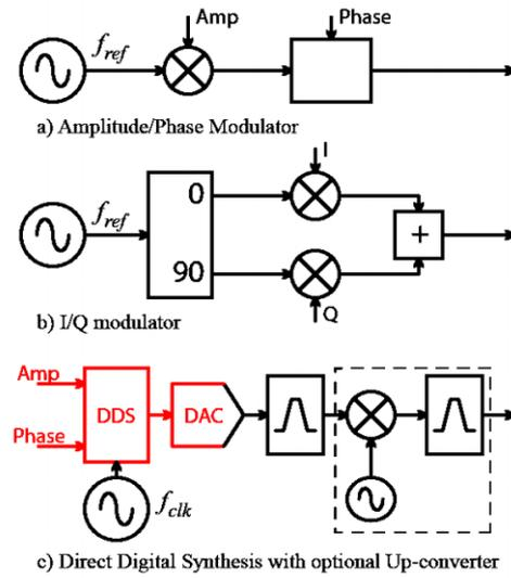
Figure 2. Different Modulation Schemes
