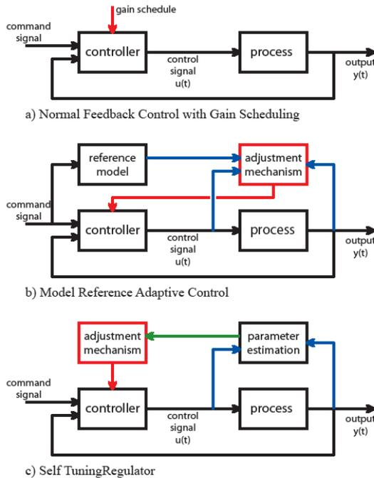
Figure 3. Block diagrams of Normal Controller and 2 types of Adaptive Controllers
