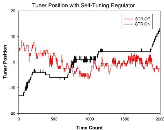
Figure 5. Performance of ISAC 2 Tuner with Self-Tuning Regulator
