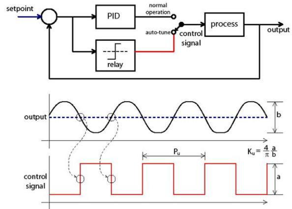
Figure 4. Auto-Tuning PID controller using Relay Method
