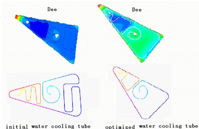
Figure 5: Water cooling tube optimization of Dee
