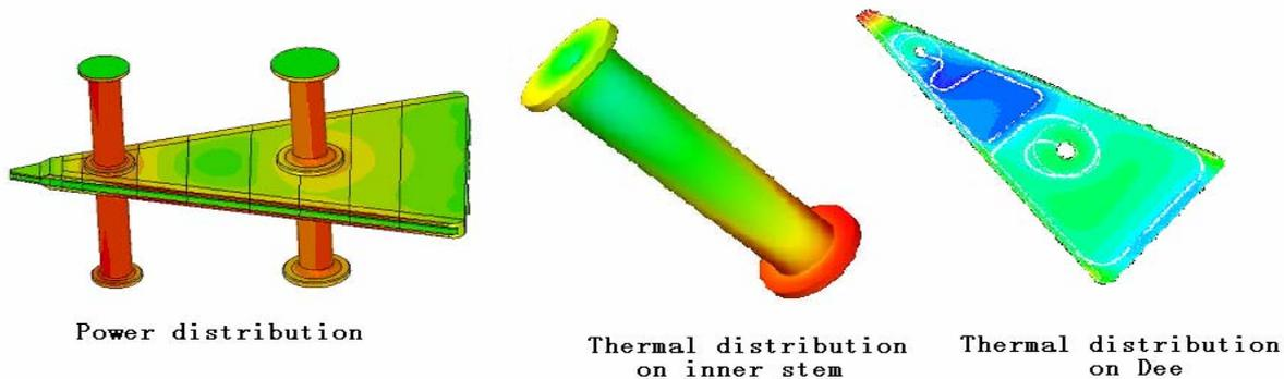
Figure 3: Thermal distribution of inner stem and Dee
