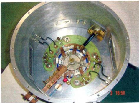
Figure 6: Input circuit (assembled) for amplifier
