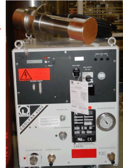
**One Stage Cryocooler at 30-50K**
