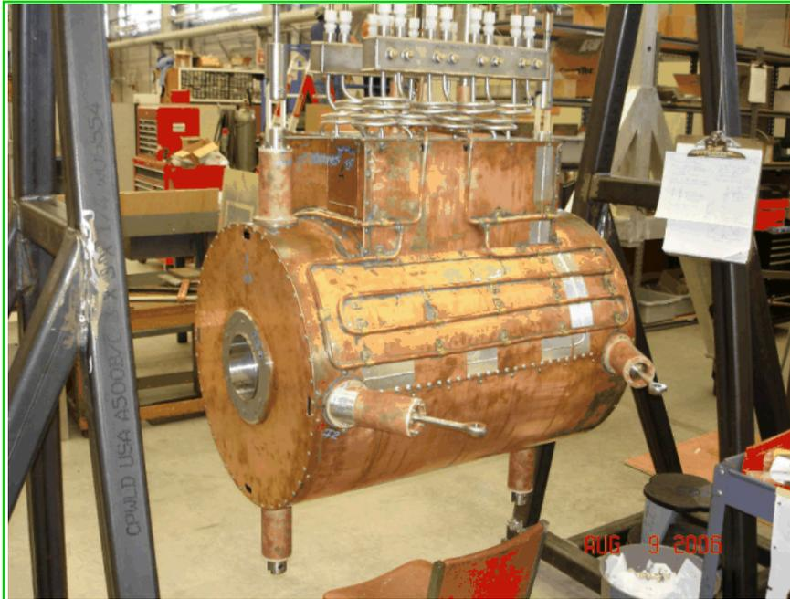
**The assembly of the SuSI magnet liquid nitrogen thermal shield.**
