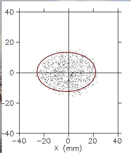
Beam spot in viewer (just after dipole)
