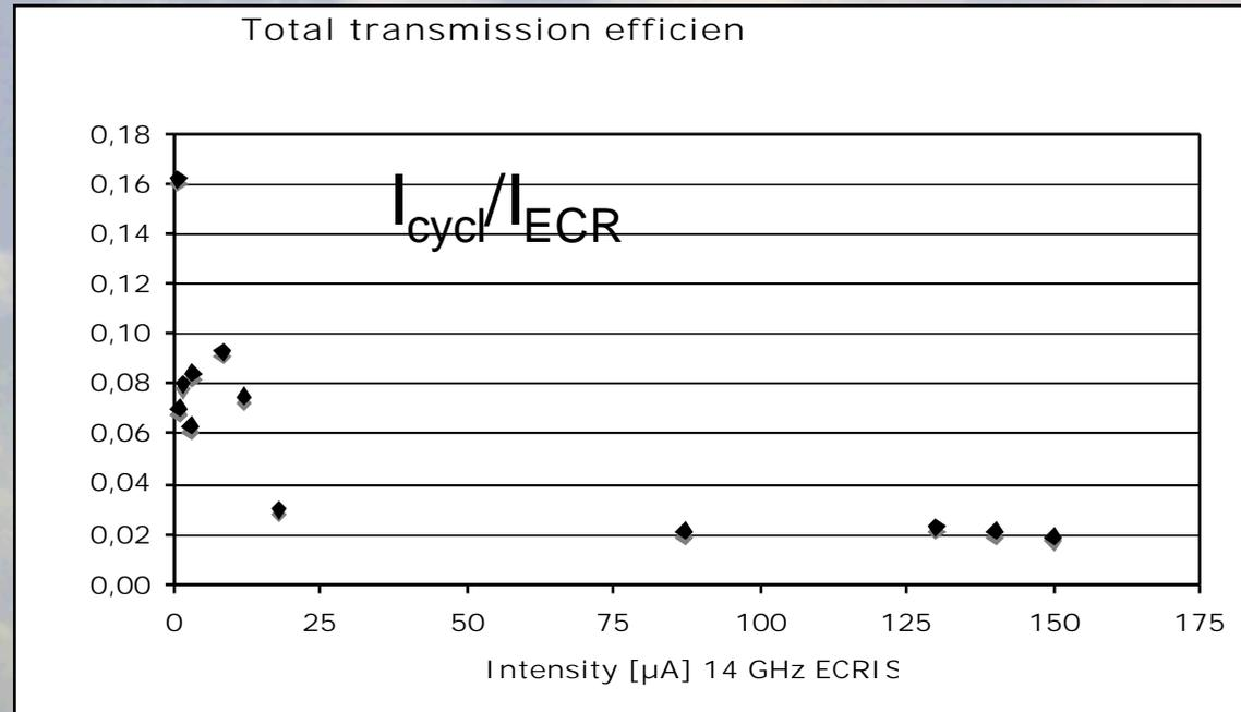
Transmission efficiency decreases when the beam intensity from the ECRIS increases!
