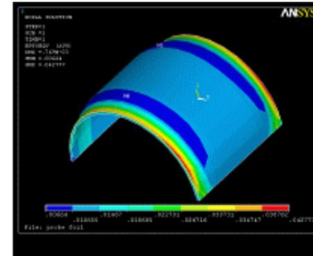
Von Mises total strain contour result at 800K
