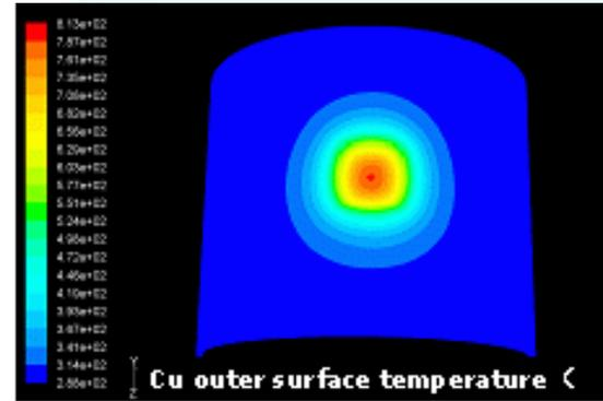
Generated heat source =  $3 \times 10^{10} \text{ W/m}^2$
