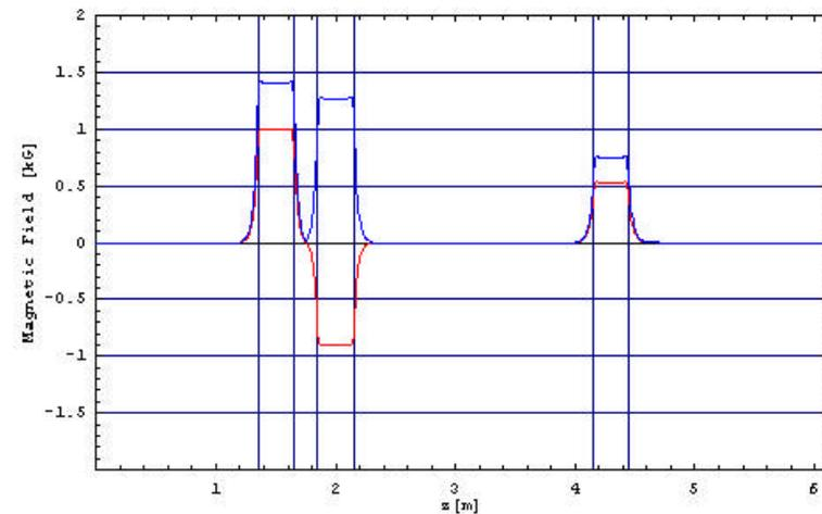
Magnetic Field Variation through the BTL with the Q-triplet
