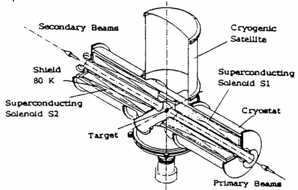
In June 2007, the second solenoid S2 of the SISSI device quenched during current rising and cannot be used since. The reasons of the repetitive quenches are still unknown (ageing, device weakness, neutron effects ...) : Short term alternative solutions are studied.
