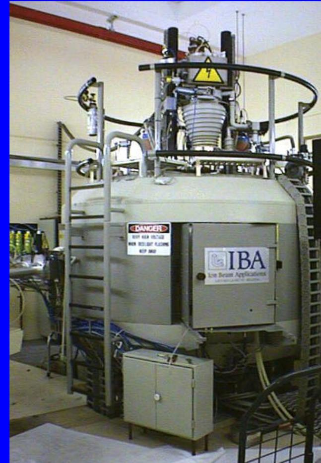
The 30 MeV H<sup>-</sup> (Negative Ion) Medical Cyclotron
