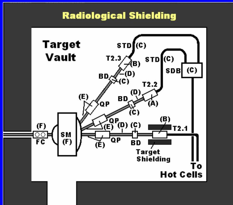
Highlighting the locations of neutron fluence measurement using Cobalt activation pellets:
