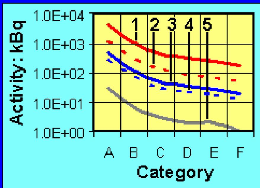
Thermal neutron induced activities of  $^{51}\text{Cr}$  (1),  $^{65}\text{Zn}$  (2),  $^{65}\text{Cu}$  (3),  $^{55}\text{Fe}$  (4) and  $^{59}\text{Fe}$  (5) generated in 1 year in 1 kg aluminium specimens (Type 5083) placed at selected areas in the target vault designated by the area categories A, B, C, D, E, F.
