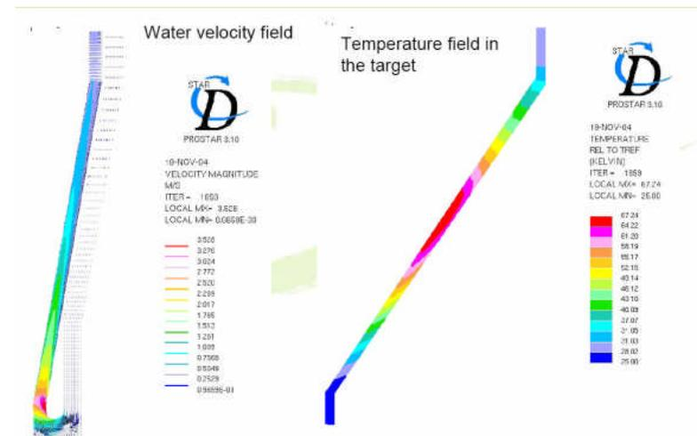
The final design was optimised for maximum activation yield (**with thermal and epithermal neutrons**) of Ho and Re in the irradiation channels
