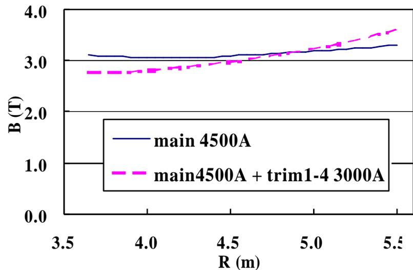
Main Coil: Bending power over the acceleration region.
