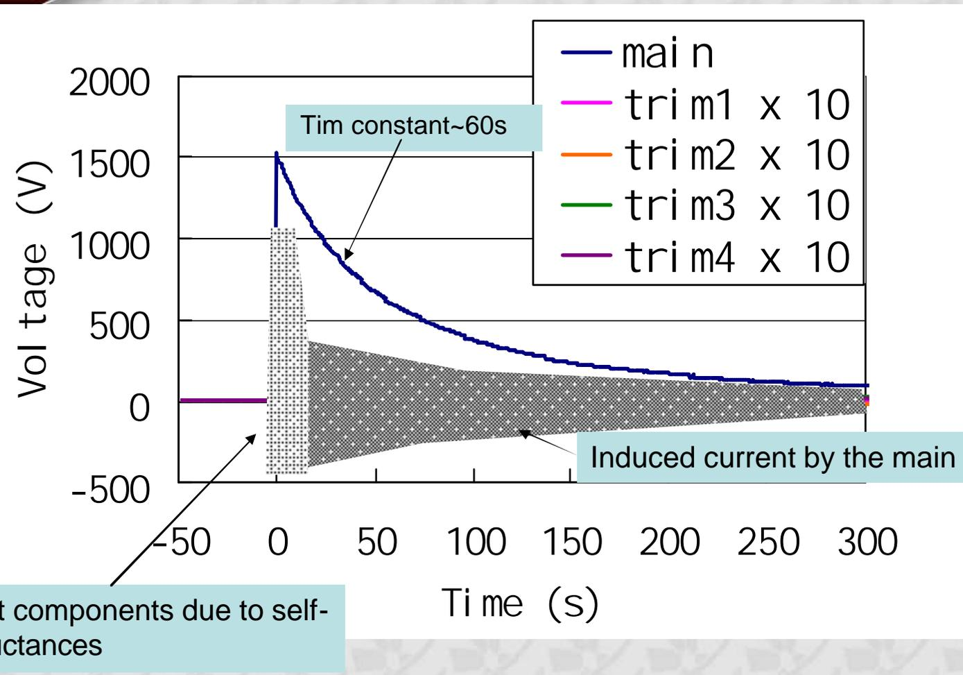
**All the coils were safely shut down even in emergency.**
