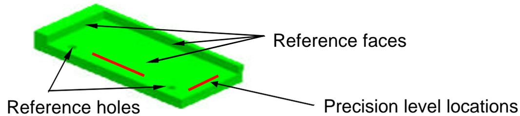
Survey plates under magnets with holes that take the laser tracker reflector spheres
