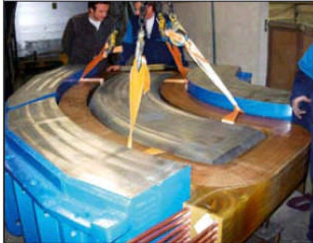
Figure 2: One 23.5-ton half of the 90 degree magnet being prepared for shipping. The 1.9 ton coils are of conventional design and could be manufactured and test assembled into the iron yoke without any major problems arising.
