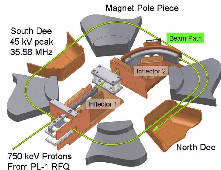
**Redesign of the Injector Cyclotron Central Region for optimal inflection onto the first orbit.**
