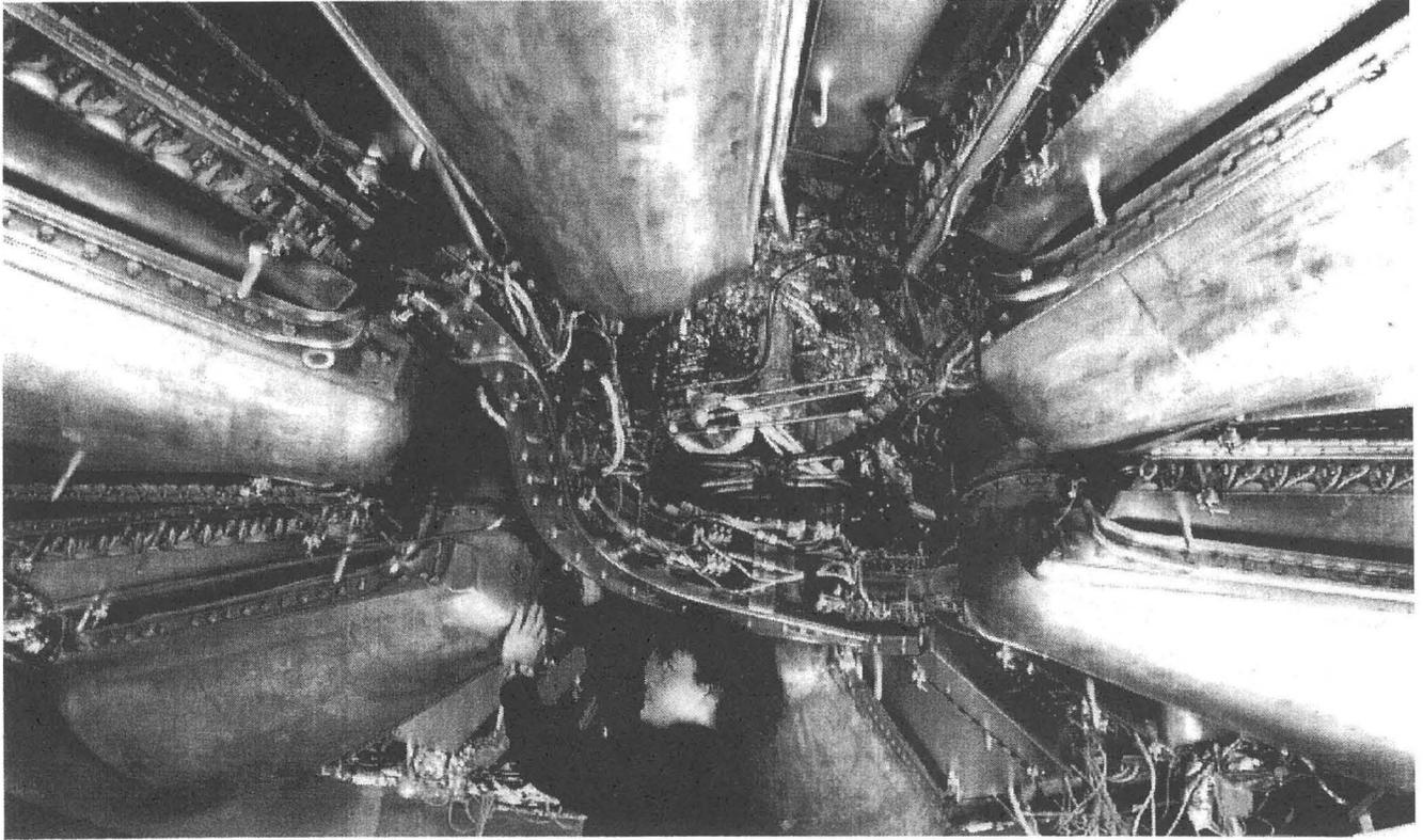
Figure 10: View from below into the Tritron cryostat with the complete machine assembled. The beam comes from the upper left corner and is injected by three channel magnets, positioned on the double-curved support above the lady.
