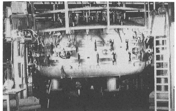
Figure 9: The Tritron cryostat. All connections are made through flanges on the upper half. The lower part can be removed.
