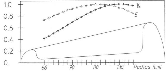
Figure 8: The radial characteristic of the amplitudes of the electrical field  $E$  and voltage  $V_0$  of the cavities.
