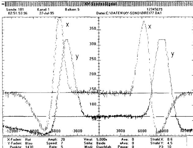
Figure 11: Typical position probe signals, taken at the end of the first turn with an injected beam current of  $\approx 10$  nA. The beam is centered rather well in the radial direction, however it is some mm above the plane of symmetry. The right part of the y-signal is cut because of overflow. The cooling rate is less for the y-filaments because of their length due to the tilt.
