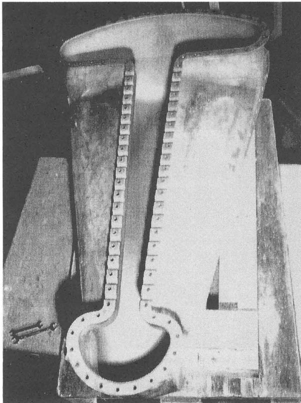
Figure 7: Two cavity halves before being screwed together in the horizontal plane of symmetry. The upper half is hanging on the supporting platform. The view is from below. No special clean room conditions are needed!
