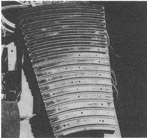
Figure 4: Lower half of a magnet sector, seen from above.
