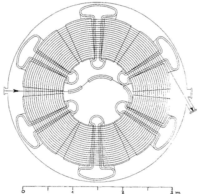
Figure 2: Horizontal cross section of the Tritron. The diameter of the vacuum vessel is 3.6 m.
