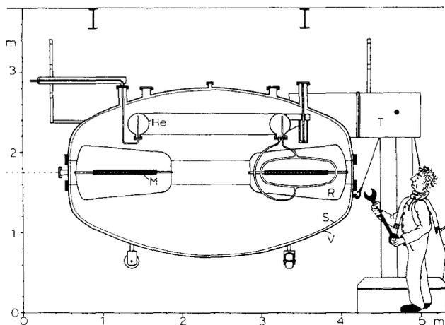
Figure 1: Cross section of the Tritron cryostat. V: vacuum vessel, S: 80K-shield, M: magnet sector, R: rf-cavity, He: helium reservoir, T: support.
