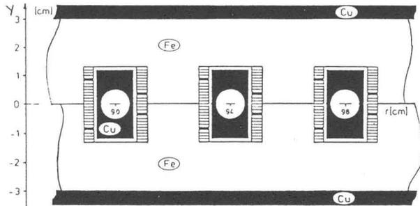
Figure 3: Radial cross section of three channel magnets.
