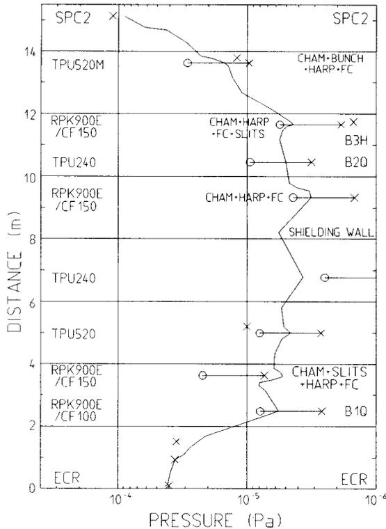
**Figure 4:** The pressure distribution in the beamline vacuum system from the ECR source to SPC2.
