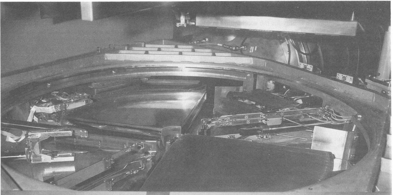
**Figure 5:** View of the interior of the injector cyclotron for polarised and heavy ions. Two of the slits, axial on the left and radial/axial on the right are visible. On the left the diagnostic harp and one differential probe can be seen. On the outer circumference some of the extraction elements, a magnetic channel on the left and the electrostatic channel on the right, can also be seen.
