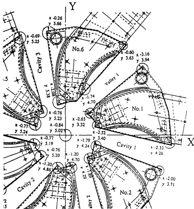
Figure 8: Status of the movement of the ring cyclotron by an earthquake.
