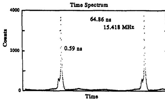
Figure 1: Time width of the extracted beam from the injector
