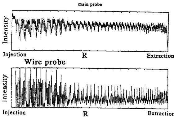
Figure 5: Acceleration beam current and turn pattern measured by an integral and a wire probe.
