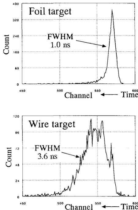
Fig. 6 : Time spectra measured with the foil target and the wire target at the collection voltage of  $-4$  kV for 260 MeV  $^{20}\text{Ne}^{7+}$  beam. The values of FWHM were evaluated on the assumption of the Gaussian distribution.
