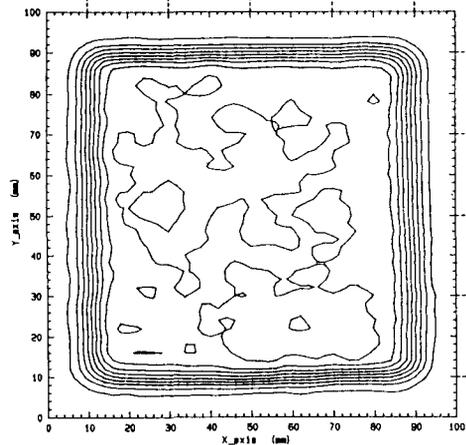
Fig. 5 : An example of fluence distribution of 175 MeV  $\text{Ar}^{8+}$  beam measured by CTA film dosimeters after modification of the beam scanner.
