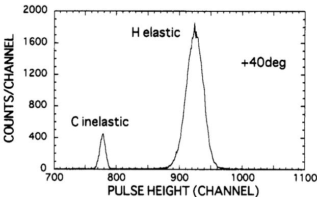
Fig. 3: Pulse height spectrum at an scattering angle of 40 deg. for a nominal 10 MeV proton.
