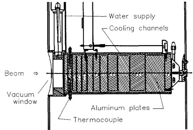
Fig. 4. The 500 MeV 200  $\mu$ A Beam Stop.
