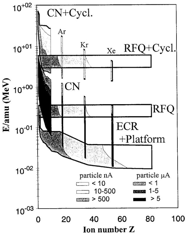
Figure 2: Ions and energies available at ISL. With the two injectors running either as stand-alone machines or in combination with the cyclotron a broad range of ions and particle energies are offered at ISL.
