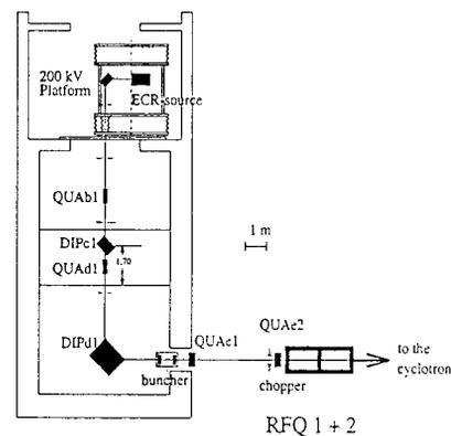
Figure 3 : Injector assembly
