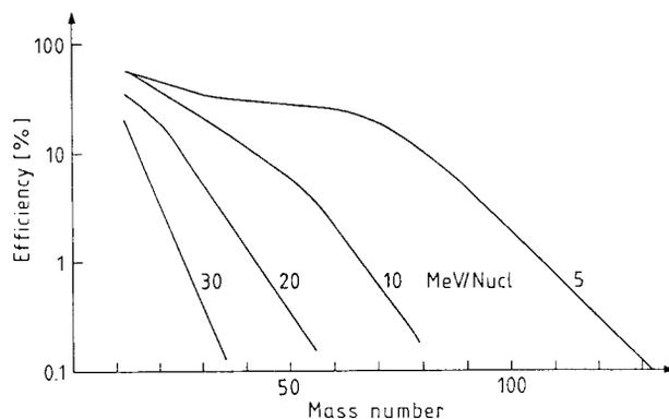
Figure 1: Stripper efficiencies for beams with different energies extracted out of the cyclotron versus ion mass.
