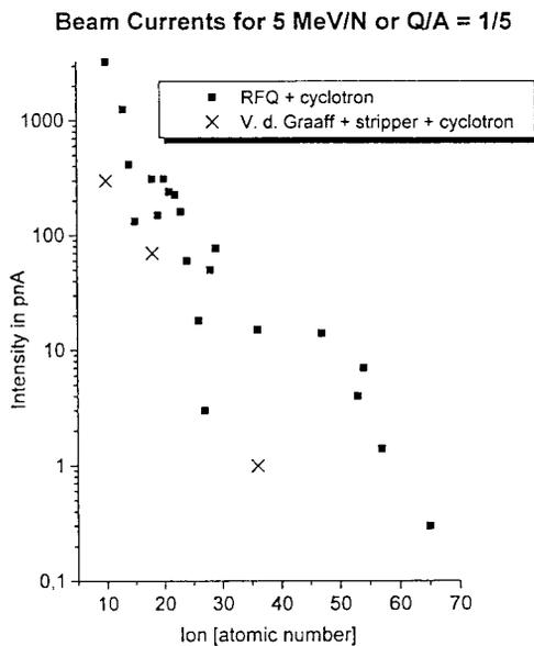
Figure 2: Intensities of ion beams with an energy of 5 MeV/amu out of the cyclotron for 2 different injectors versus atomic number (for the RFQ injector a total transmission from the source to the experiment of 10 % is assumed).
