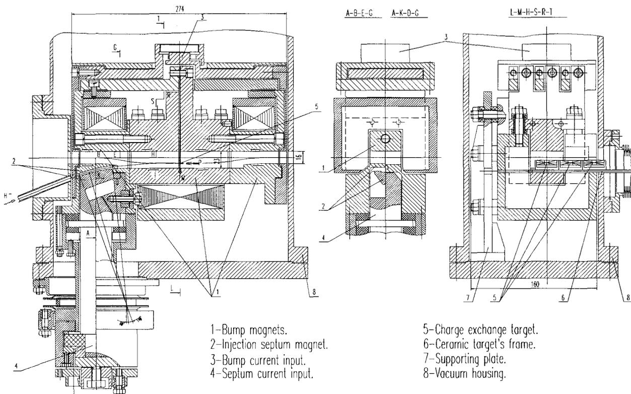
**Figure 7 :** Charge exchange injection system into compact proton synchrotron.
