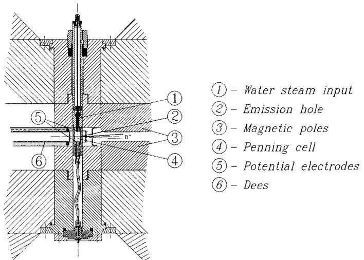
**Figure 3 :** Cyclotron central part azimuthal cross-section (internal injection version).
