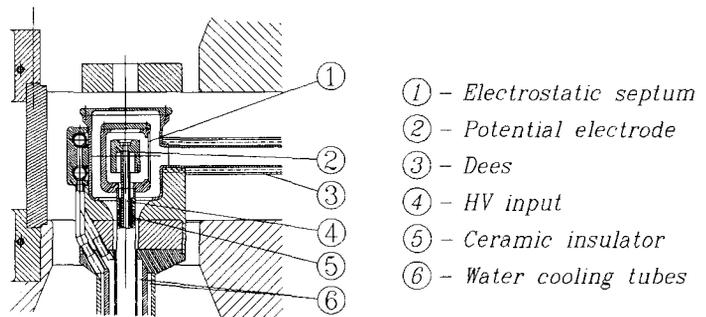
**Figure 5 :** Electrostatic septum and high voltage input cross-section.
