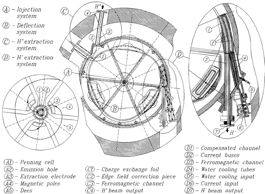
**Figure 4 :** Cyclotron injection (internal version) and extraction systems
