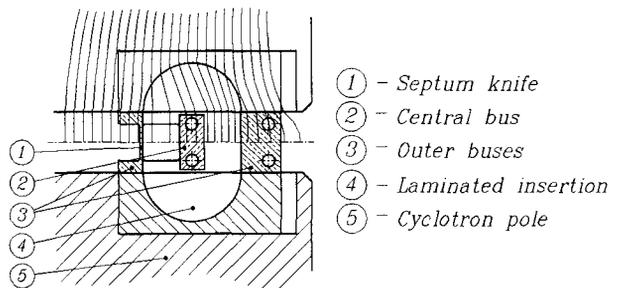
**Figure 6 :** Pulse extraction system cross-section and magnetic flux
