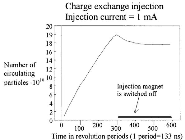
**Figure 9 :** Dynamics of particle accumulation with injection time of  $40\ \mu\text{s}$
