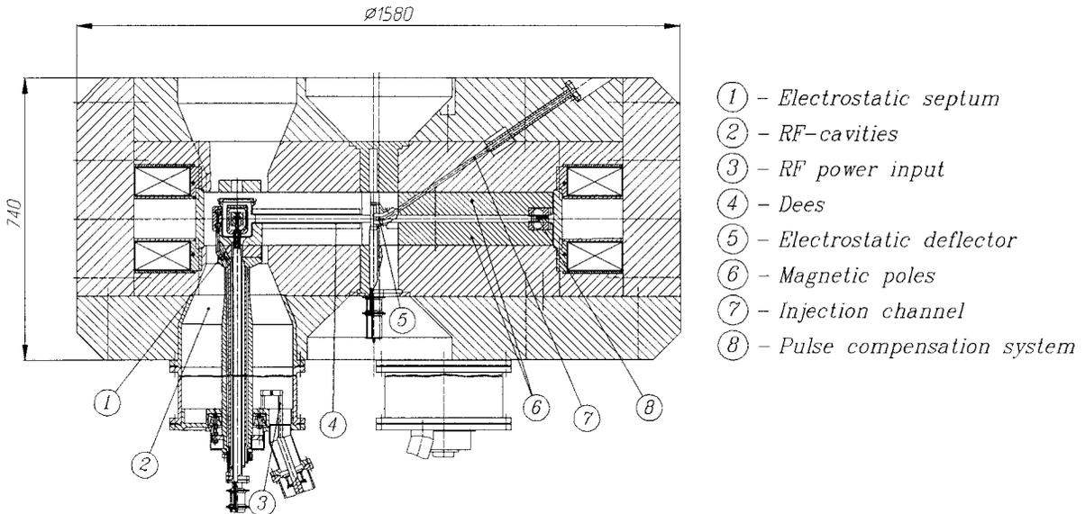
**Figure 2 :** Azimuthal cross-section of cyclotron (external injection version).
