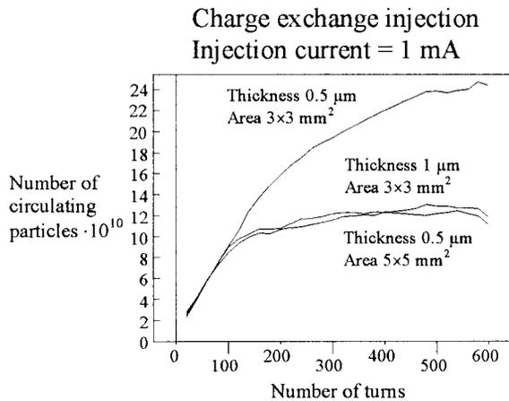
**Figure 8 :** Dynamics of injection with various parameters of charge exchange target.
