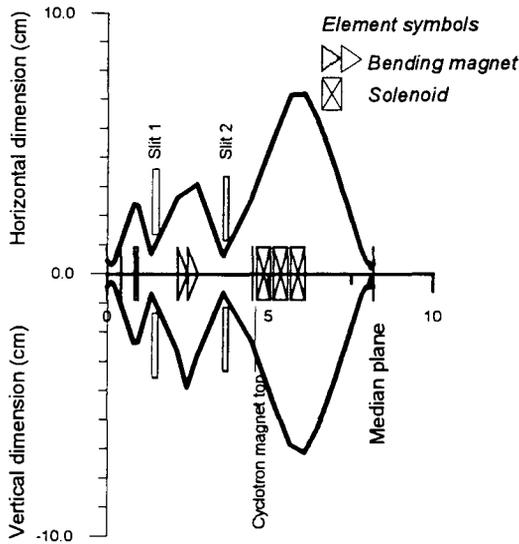
Figure 6: The beam environment in the beam axial injection system of U400M.
