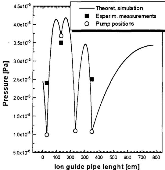
Figure 7: The distribution of pressure in the axial injection system of U400M.
