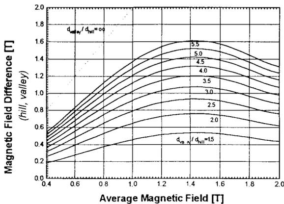
Figure 2: The dependence of  $\Delta B = B_{\text{hill}} - B_{\text{valley}}$  on  $\langle B \rangle$  and  $d_{\text{hill}}/d_{\text{valley}}$ .
