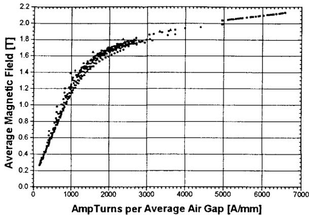
Figure 1: The dependence of  $\langle B \rangle$  on the excitation of the magnet  $0.5 \times (d_{\text{hill}} + d_{\text{valley}})$ .
