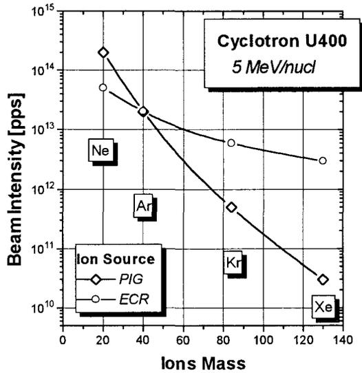
Figure 3: The expected increase of intensity in the complex ECR+U400 for an ion energy of 5 MeV/u.
