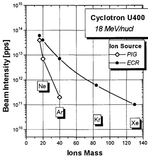
Figure 4: The expected increase of intensity in the ECR+U400 complex for an ion energy of 18 MeV/u.
