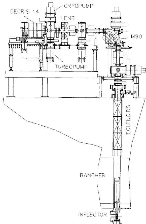
Figure 5: The scheme of the beam axial injection into the U400M.
