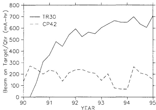
Figure 5: Total charge delivered on target each quarter by the TR30 and CP42 cyclotrons located at TRIUMF, and owned by Nordion Int.
