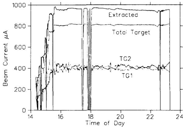
Figure 6: Initial high current beam test with the TR30 cyclotron
