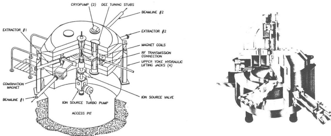
Figure 1: Schematic views of the TR30 cyclotron (on left) and the CYCLONE 30
