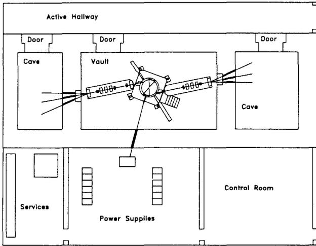
Figure 3: A typical layout for a third generation cyclotron being used for isotope production
