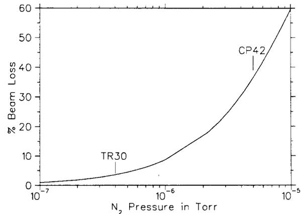
Figure 2: Beam losses due to gas stripping as a function of pressure for a 30 MeV cyclotron.
