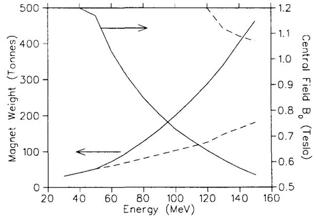
Figure 7: Required Magnet Sizes as a function of Energy for a  $H^-$  Cyclotron. The electro-magnetic stripping losses have been constrained to be less than 2% on the solid curves.
