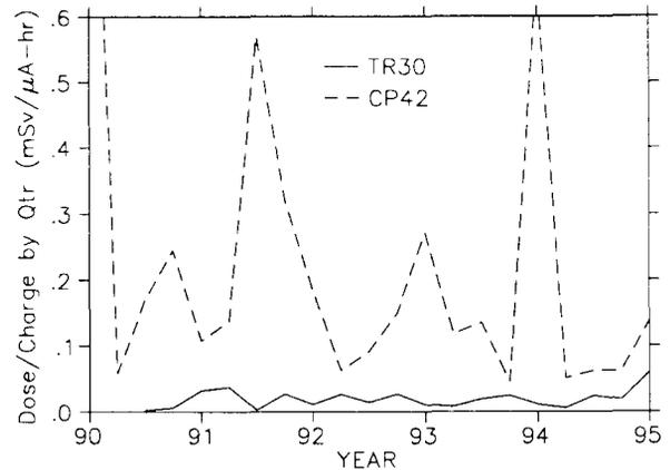
Figure 4: Accumulated personnel radiation dose, by quarter for the TR30 and CP42 cyclotron. Major repairs lead to the large spikes in the CP42 curve.
