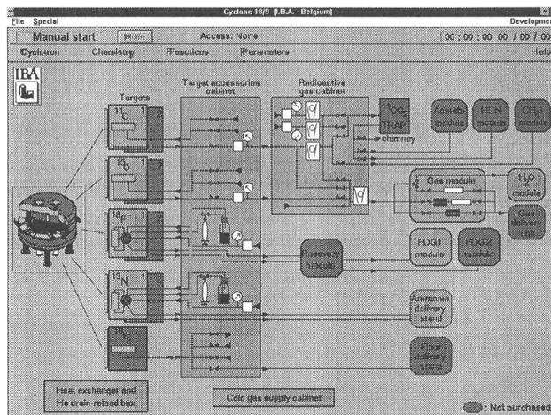
Fig. 2 : Central Flowchart for the Control of the PET System
