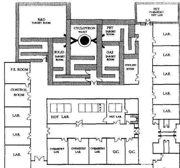
Fig 1. Layout of the Cyclotron facilities
