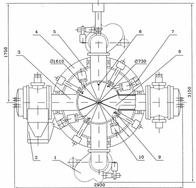
Fig. 1. Plan view of the RIC-10 cyclotron: 1. Diffusion pump. 2. RF generator. 3. Vacuum chamber. 4. Electromagnet. 5. Main coil. 6. Beam probe. 7. Hydraulic lift. 8. Dee. 9. Stripping foil. 10. Target
