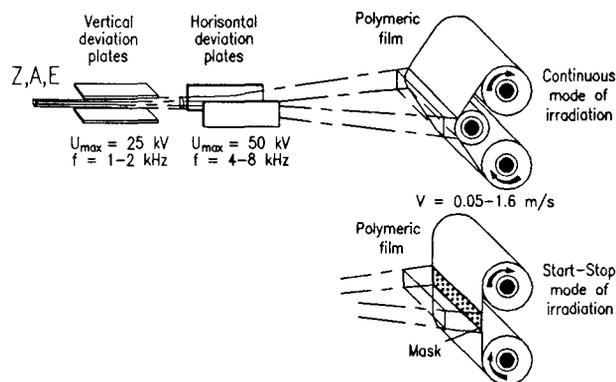
Fig. 5: Plan of the irradiation facility using a scanning beam from the U-400 cyclotron at FLNR JINR.
