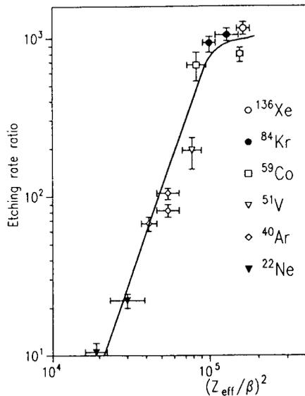
Fig. 6: Track etch rate to bulk etch rate ratio as a function of the bombarding particle parameter [8] (here  $Z_{\text{eff}}$  is effective charge of an ion and  $\beta$  is its relative velocity).
