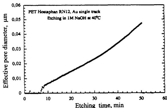
Fig. 3: Effective pore diameter as a function of etching time for the sample with a single heavy ion track
