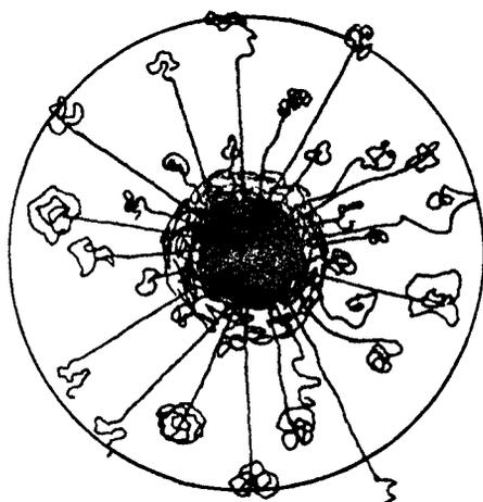
Fig. 1. Schematic model of a heavy ion track (cross-sectional view). The core and penumbra radii are shown [12].
