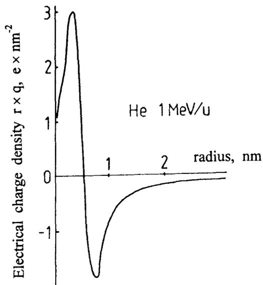
Fig. 2: Transient ( $10^{-14}$  -  $10^{-13}$  s) electrical charge distribution in a heavy particle track in insulator (after A.G.Weisburd and D.I.Weisburd [13])
