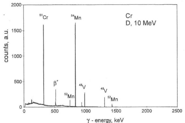
Fig. 2:  $\gamma$ -spectrum obtained from the chromium substrate by activation with 10 MeV deuterons.
