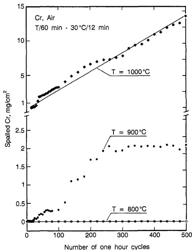
Fig. 3: Spallation behaviour of chromium due to thermal cycling from various maximum temperatures to ambient temperature.
