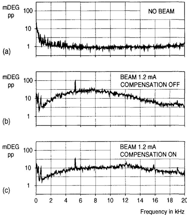
Figure 6 : Effect of beam load compensation on flat-top cavity phase spectra
