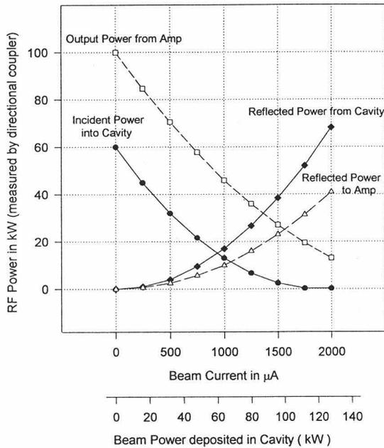
Figure 3: RF power levels as a function of beam current, showing extrapolated range to 2mA
