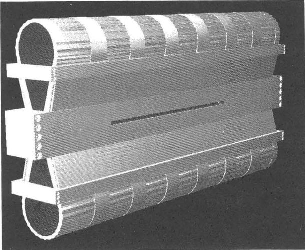
Figure 11: 150 MHz test cavity (1:3 scale model)
