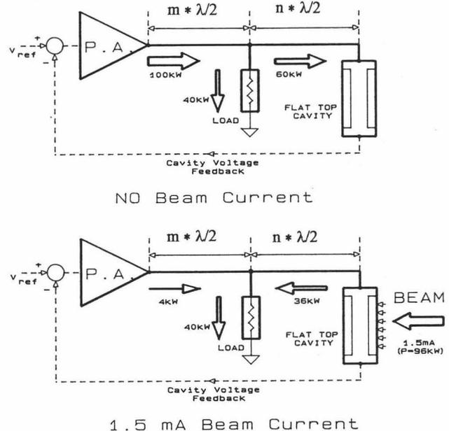
Figure 2: Symbolised RF energy flow at 0 and 1.5 mA beam levels
