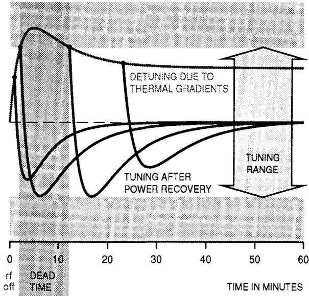
Figure 10: Cavity tuning behaviour, after RF-drive interrupt; for 4 different start delays. The starting-point curve shows the strong influence of thermal gradients in the cavity walls.
