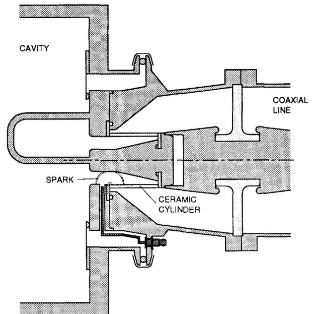
Figure 7: Coupling loop cross-section, with spark detection probe
