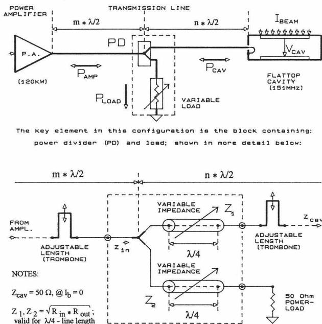
Figure 4: Schematic of the cavity loading network
