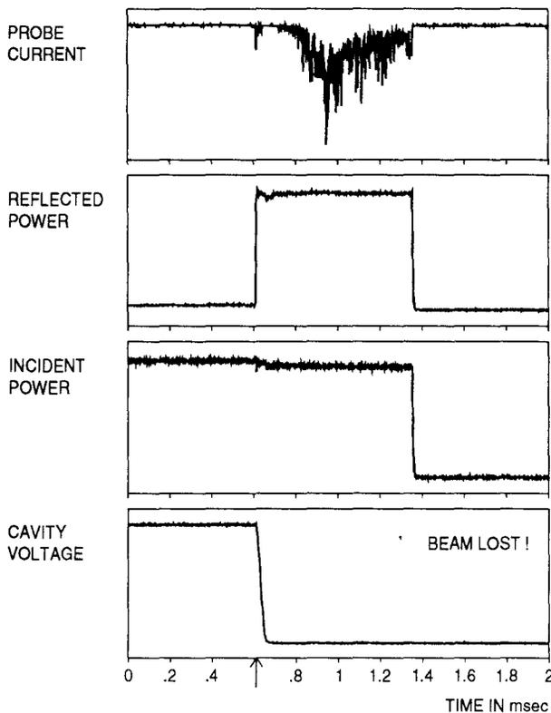
Figure 8: Timing diagram of signals from: spark detection probe, cavity voltage, and transmission line power levels; without suppression circuit.
