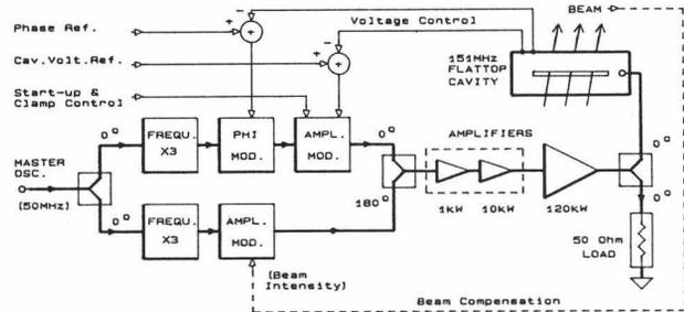
Figure 1: Block diagram of the PSI flat-top system
