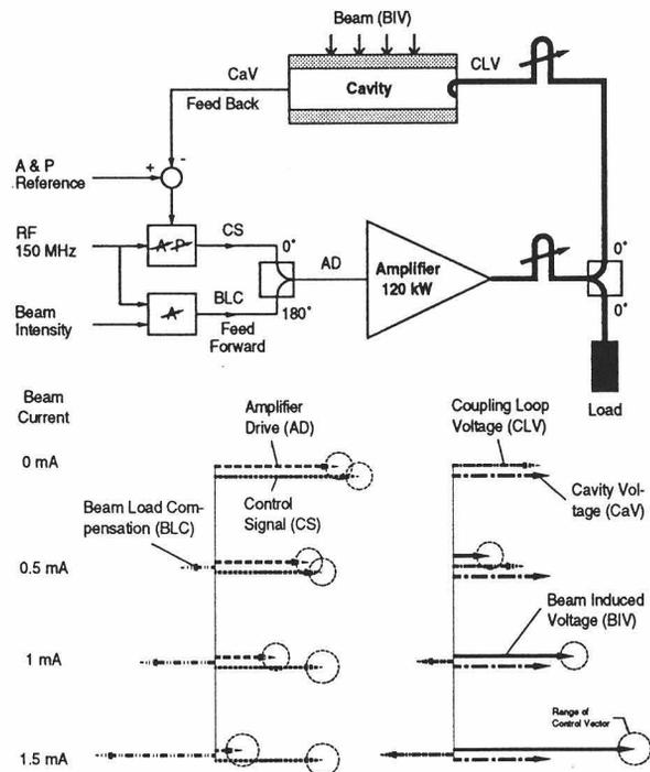
Figure 5: Phasor diagram, showing voltage phasors at different points in the system, for selected beam currents.
