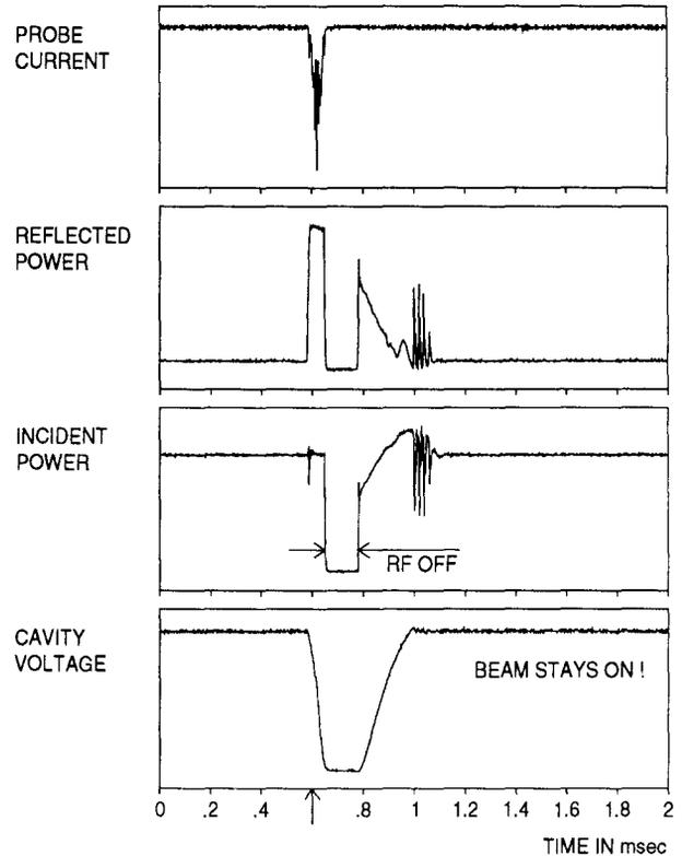
Figure 9: Timing diagram, same configuration as in fig.8, but with suppression circuit active.
