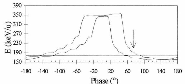
Fig. 8: Output energy as function of the phase of RFQ<sub>2</sub>.
