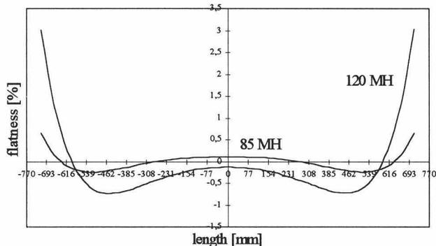
Fig. 7: Voltage distribution for highest and lowest tuner positions.
