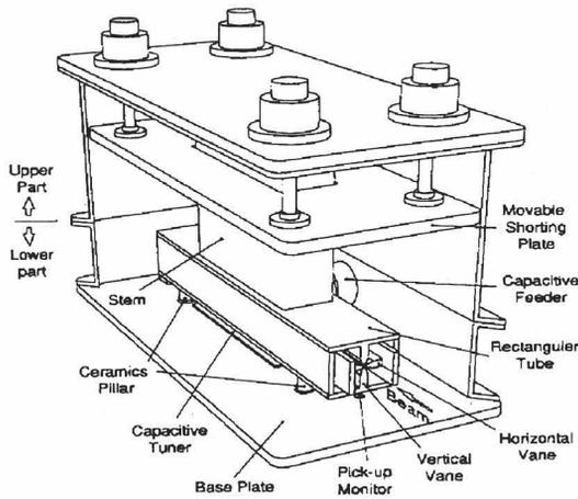
Fig. 3: Schematic drawing of the RIKEN-RFQ resonator.
