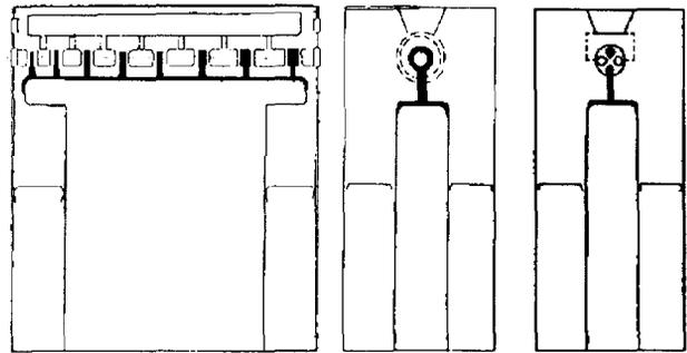
Fig. 2: Scheme of asymmetric RILAC - drift tube structure and added 4-rod-RFQ-electrodes.
