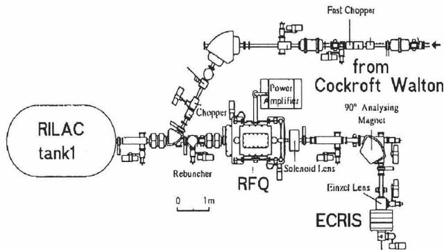
Fig. 4: RILAC-injector layout.
