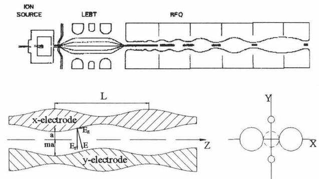
Fig 1: Scheme of RFQ-injector and modulated electrodes.
