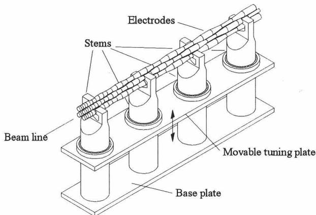
Fig. 6: Scheme of the VE-RFQ at HMI.
