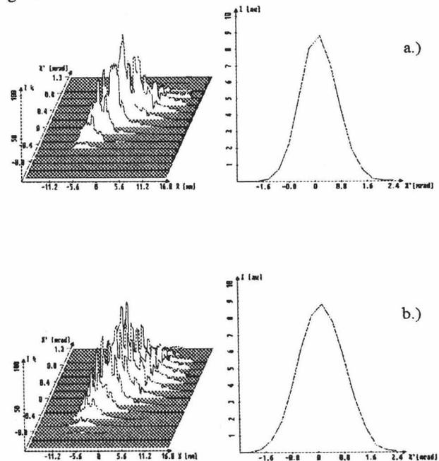
Figure 5: Density distribution in the 2-dimensional horizontal phase space and angular profile a) without and b) with stripping foil.
