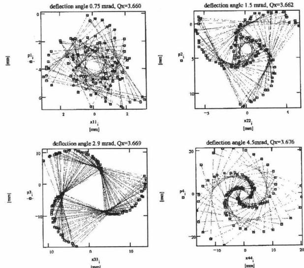
Figure 8: Transverse phase space plots for four different kick amplitudes resulting in the given deflection angles. Proton momentum is 800 MeV/c. The straight lines connect the measured data in turn.
