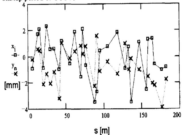
Figure 7: Narrowband measurement of the corrected closed orbit in the horizontal (x) and vertical (y) plane along the ring.
