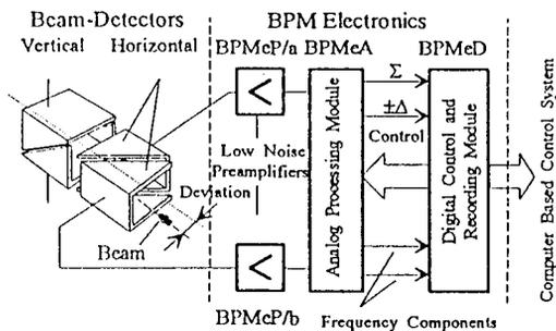
Figure 6: Beam Position Monitor Electronics Assembly.
