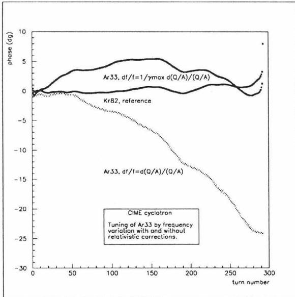
Figure 1. Phase vs turn number after frequency variation
