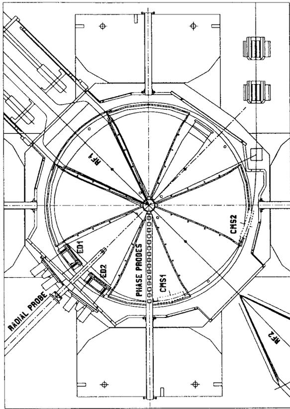
Fig. 3. CIME Cyclotron median plane
