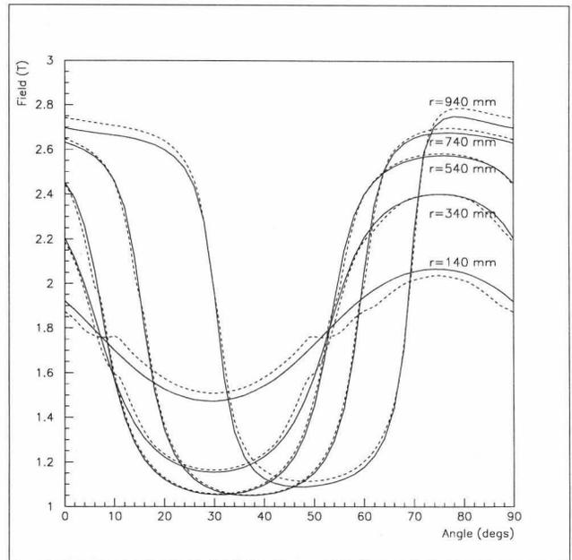
Figure 4: The measured (full) and 3-D modelled (dash) fields are in good agreement at all radii
