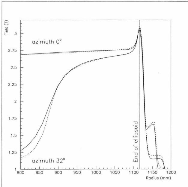
Figure 3: Comparison between measured (full) and 2-D model (dash) at 2 different azimuths on the pole featuring the gradient corrector for the initial radial edge
