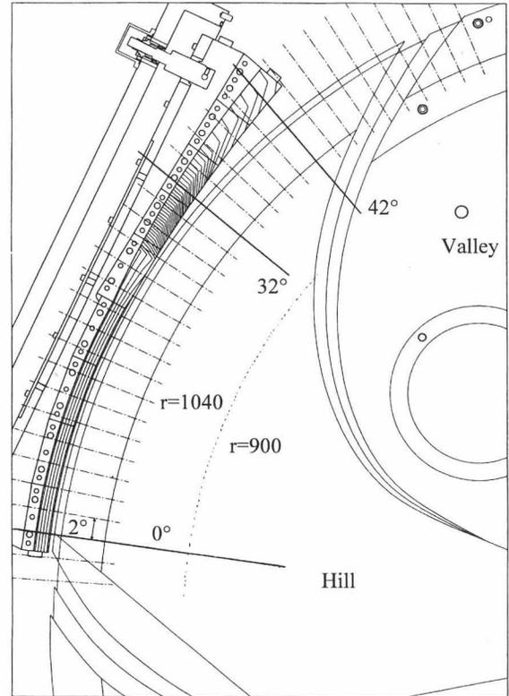
Figure 2: Top view of the pole featuring the gradient corrector
