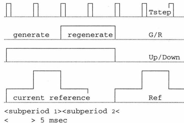
Figure 3. Timing diagram of the control and reference
