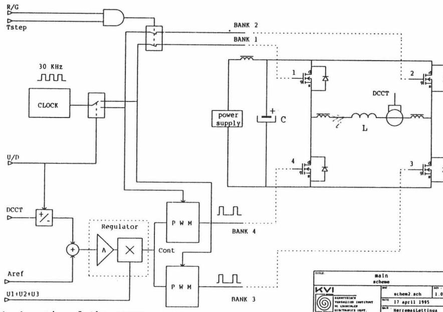
Figure 2. blockschematic of the power supply.
