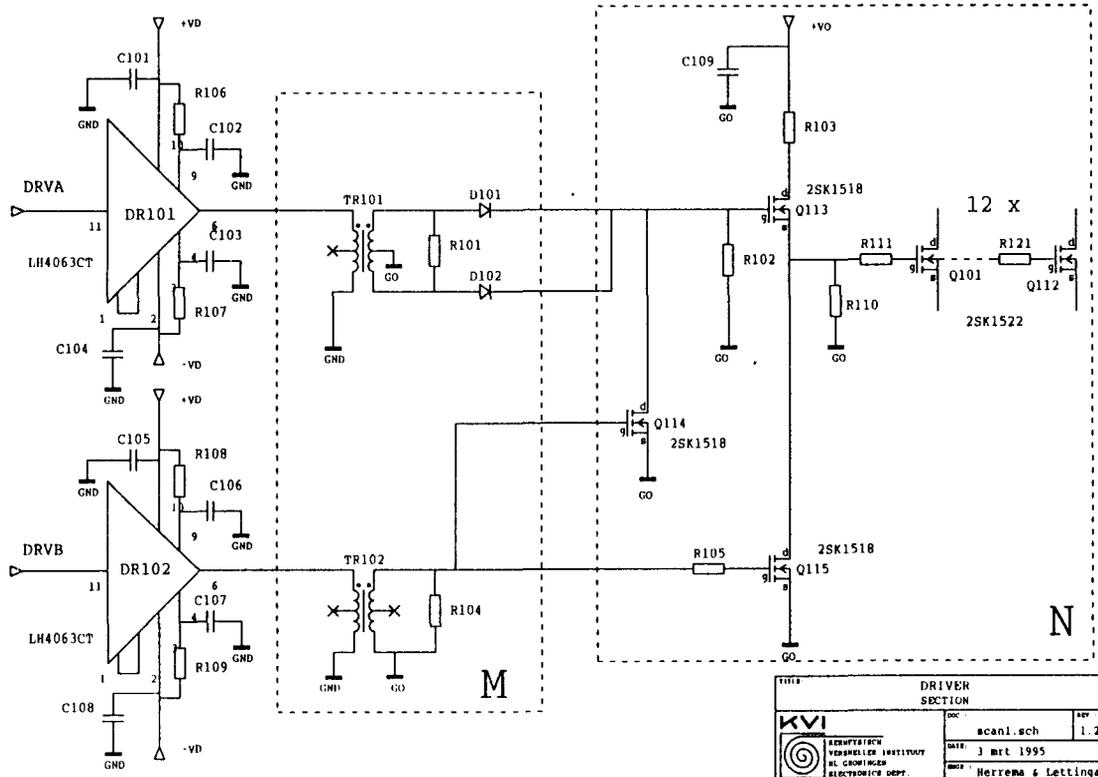
Figure 4. Circuit schematic of the fetbank control.
