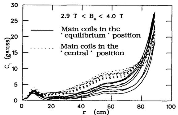
Figure 1: First harmonic measured before and after coils centering
