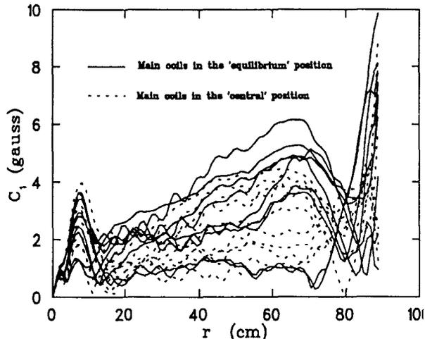
Figure 5: First harmonic measured after shim installation with the coils in the two positions
