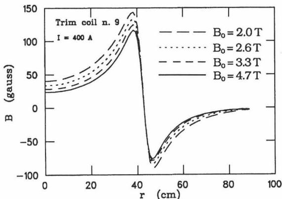
Figure 3: Trim coil n. 9 form factor at different field levels
