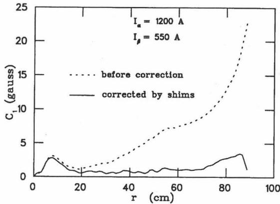
Figure 2: Effect of the shims on the measured 1<sup>st</sup> harmonic
