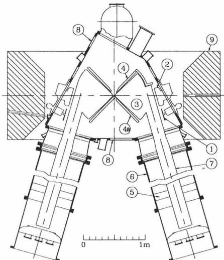
Figure 1. A top view of the SPC1 resonators, showing: (1) The main coupling capacitor, (2) the trimmer capacitor, (3) the dee, (4 and 4a) the dummy dee, (5) the short-circuit plate, (6) the outer conductor of the coaxial section, (7) the inner conductor, (8) the vacuum chamber, and (9) the magnet.
