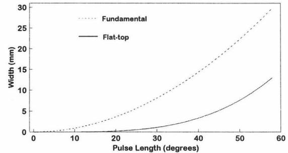
Figure 2. The increase in the beam with due to energy spread at extraction in SPC1 with and without a fifth harmonic flat-top system.
