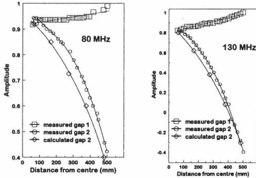
Figure 5. The measured and calculated fifth-harmonic voltage distribution along the acceleration gaps for the full-scale SPC1 resonator model at 80 MHz and 130 MHz. Gap 1 is indicated by no 4 and gap 2 by no 4a in figure 1. In the program FLATOP it is assumed that the voltage along gap 1 is constant.
