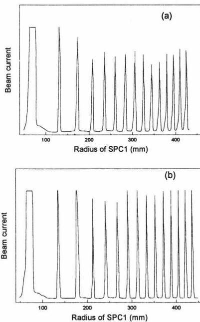
Figure 6. The beam pattern in SPC1 without (a) and with (b) the fifth-harmonic flat-top system. The beam width decreased from 12 to 8 mm at the extraction radius due to the reduced energy spread with the flat-top system for a beam intensity of 190  $\mu$ A.
