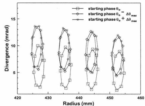
Figure 4 The calculated phase ellipses in the r-r' phase space at the of the last four turns at the extraction radius of SPC1 with the flat-top system. The three ellipses for each turn correspond to phases of  $-30^\circ$ ,  $0^\circ$  and  $30^\circ$  respectively. The turn separation between the last two turns is 4.5 mm.
