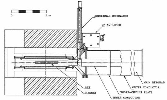
Figure 3. An additional transmission-line resonator, capacitively couple to an SPC1 resonator. The additional resonator is 1.2 meter long, and the diameter of the inner and outer conductor are 40 mm and 120 mm, respectively.
