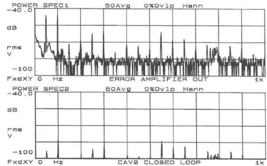
Fig. 5 - The driving and the resulting signals of the am-loop.
