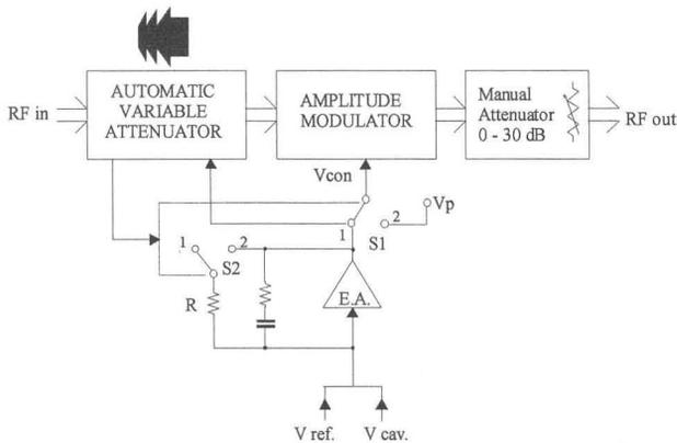
Fig. 4 - Block-diagram of the amplitude-loop.
