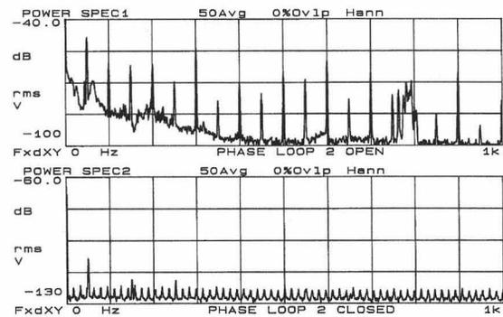
Fig. 3 - The open and closed phase-loop signals.
