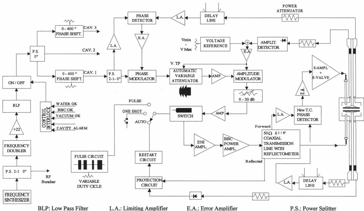
Fig.1 - Block diagram of the electronic RF-system.
