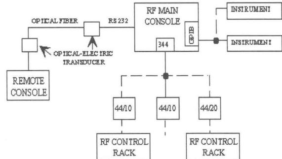
Fig.9 - Block diagram of the RF Computer-Control
